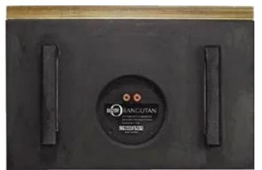
The connection panel sits on the underside, making access difficult. Spade terminals are best used here.
